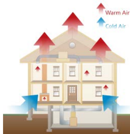
FIGURE 3: ILLUSTRATION OF STACK EFFECT IN A RESIDENCE
