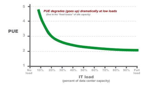
Each data center will have a higher or lower infrastructure efficiency curve – depending upon the efficiency of its individual devices and the efficiency of its system configuration – but the curve always has this same general shape.
