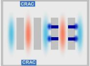
The placement of cooling units close to the servers provides the essential element that is the key to efficient cooling: short air paths. A short air path between cooling and the load enables a number efficiency and availability benefits:
