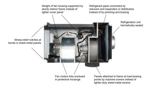
Specifically, check to see if the fan motors are fully enclosed in protective housings to prevent dust from building up. Dust that accumulates on the motors can absorb moisture, leading to corrosion or electrical shorts.
