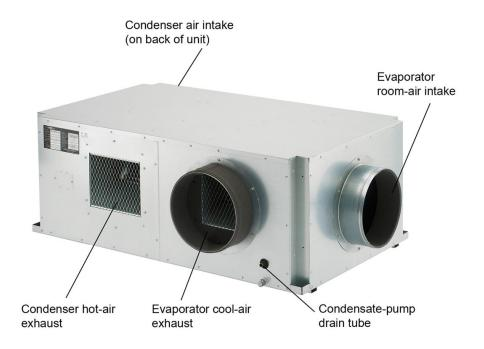
As with conventional systems, cold refrigerant flows through copper tubing from the condenser to the evaporator coil. A fan blows over the coil, pushing cold air out. A second fan pushes hot exhaust air out through a flexible duct, which is usually directed into the crawl space above a drop ceiling.
